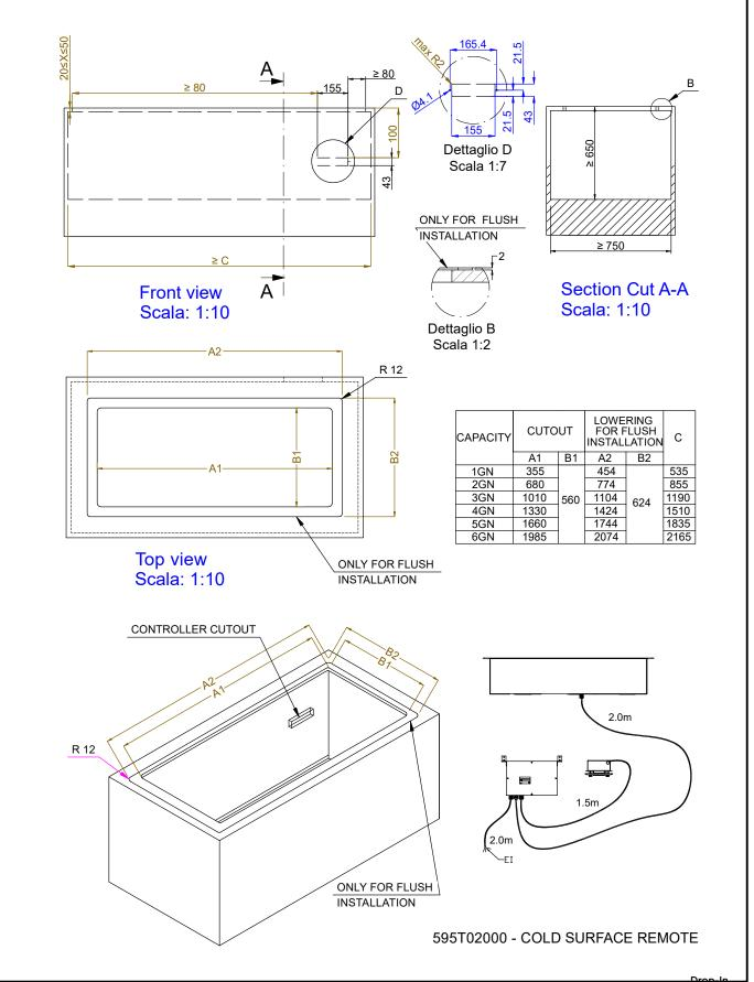
Drop-in remote refrigerated quartz surface (4 GN container capacity)
